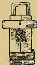
Fig. 33.—Sight on an ancient cross-bow in Tower of London, showing Peep Sight and Lateral Sliding-bar Wind Gauge.
